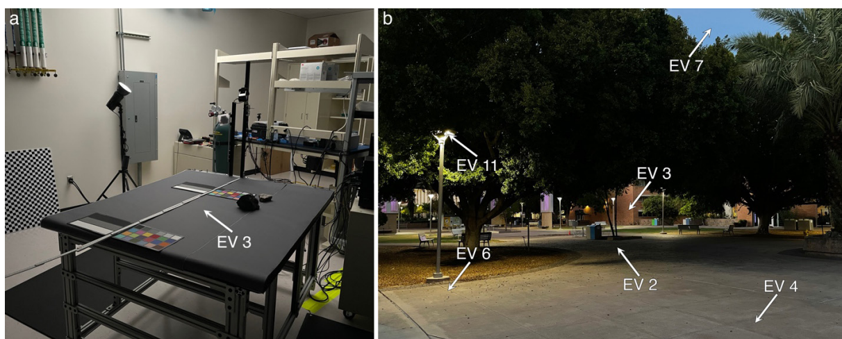
Fig. 10. Earth analogues for PSR lighting. (a) Lab setup for testing the imaging system for Grace at potential PSR luminance levels. Light aimed at ceiling in an otherwise-unlit room was adjusted until center of table was at the target EV. (b) Outdoor twilight scene (looking northeast with a building immediately to the west, clear sky, 12 minutes after sunset); reflected luminance was measured at marked locations. Image exposure was adjusted at time of acquisition until the preview qualitatively matched the perceived appearance of the scene. Note that all of these surfaces are more reflective than mature regolith, so there would likely be more ambient light in a crater that has the same luminance as this scene. PSR, permanently shadowed region; EV, exposure value.
