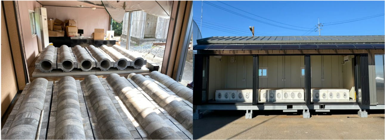
Fig. 2. Disassembly of the Daejeon neutron monitor (NM) (left) and the assembly of the NM at Mt. Gamak (right).
