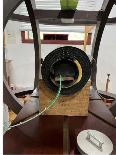
**Fig. 8.** Photograph of the shielding can and fluxgate magnetometer (FGM) for noise test.
