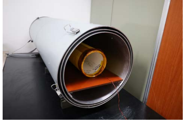
Fig. 5. The magnetic shielding case and test solenoid.
