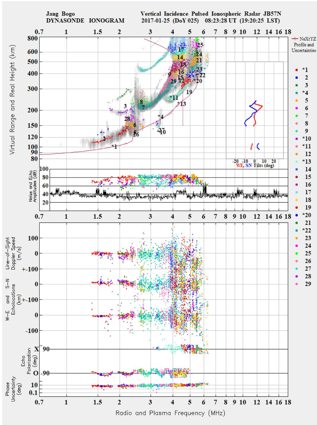
**Fig. 5.** Ionogram image (top) in the standard Dynasonde presentation format. Also shown at the bottom panel are Doppler, echolocations, polarization, and error parameter. Echo group range versus radio frequency appears in the logarithmic scales. Colored dots in the figure denote echo traces. The inset of the top panel shows the meridional (blue) and zonal (red) local tilt angles of each constant plasma density plane.
