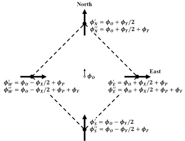
**Fig. 6.** Schematic representation of the Dynasonde receiving array and echo phase information adopted from Wright & Pitteway (1979b). Arrows at corners of the square array represent dipole lengths and directions. Primed phases are measured at  $f$  and double primed phases at  $f + \Delta f$ . Adopted from Wright & Pitteway (1979b) with AGU permission policy.
